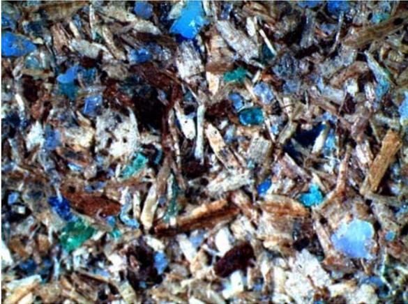
**Fig. 9** Surface of particle board containing 30% PET.
