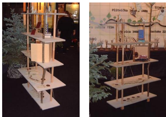
Figure 3: The shelving unit produced from longitudinally connected turned elements by the method of welding, international fair Ambianta 2012, Zagreb
