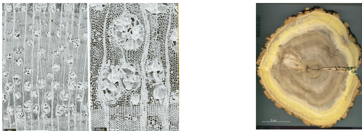
Fig. 1.: Microscopic (left) and macroscopic (right) structure of Robinia
