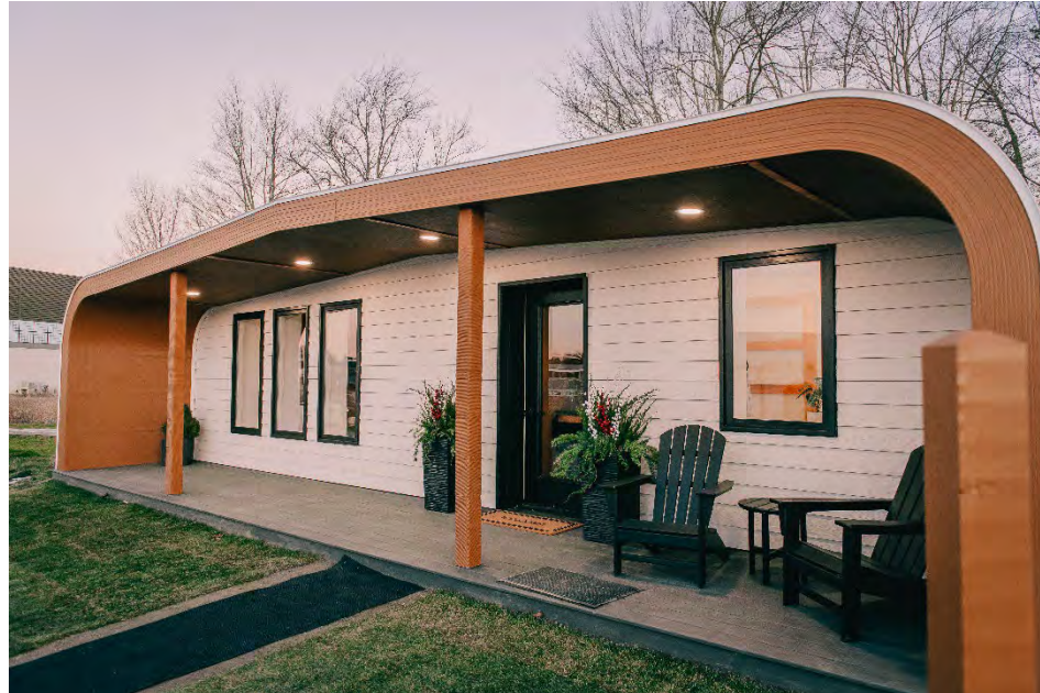
3D printed house, BioHome3D, made from wood and biobased polymer at University of Maine
