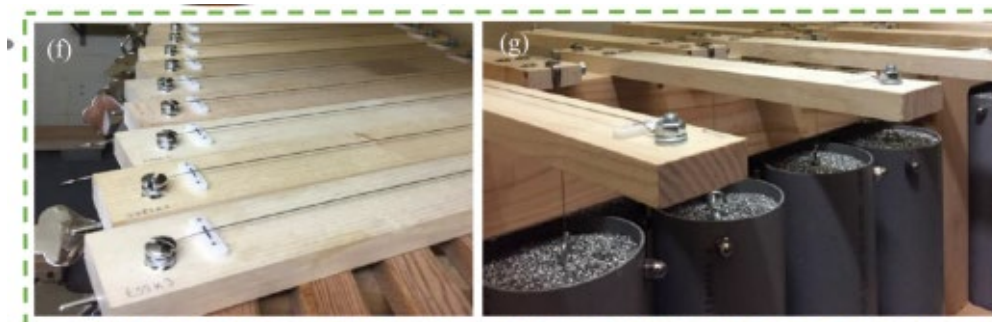
Fig. 1: Tuning-key (left) and weight-loaded tension set-up (right). From [1].
