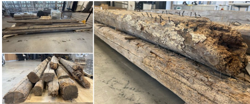
Fig. 1: Reclaimed timber beams recovered from a former Servite Monastery in Koper, Slovenia.
