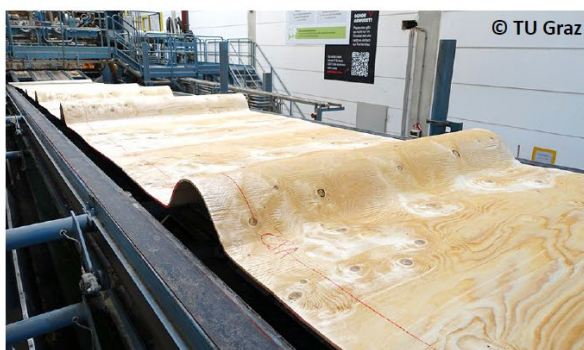
“rethink_LT_processing”, peeling process: t = 10\text{ mm}
