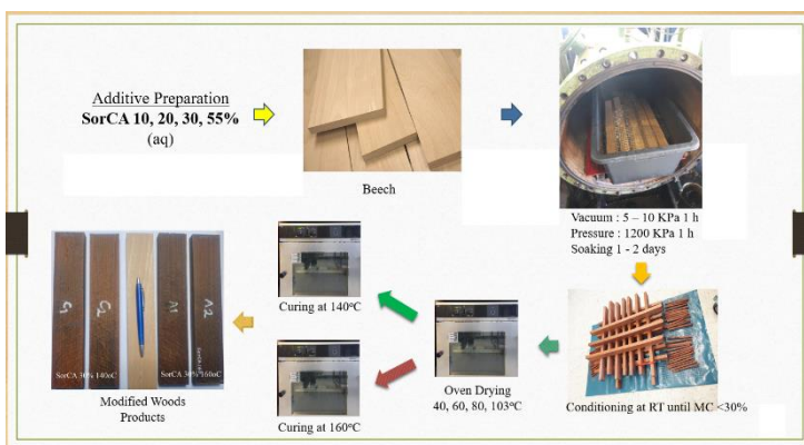
Figure 2 Polyesterification of sorbitol-citric acid (left) and wood modification process conducted in the second section of the study (right).
